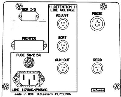
ADJUST: The three pin plug from the pitch drive motor is plugged into this socket.
