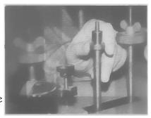
Adjust the height of the pitch drive motor using the two legs on the base of the pitch drive motor housing so that the flex shaft is parallel to the coiler. Fasten the flex shaft to the pitch drive motor.
