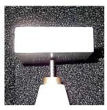
Using the probe holder, target the 1/8" probe tip against a flat spot on the coiler to simulate a spring. Make sure the tip is flush on the spot. Back the micrometer out .065" as the standoff distance.
