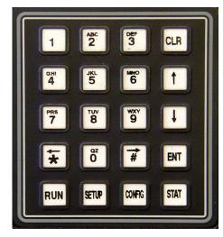
to the right, while filling the left with '0'. The '0' thru '9' keys will shift the number one place left and insert the digit pressed. The up and down arrow keys increase and decrease the number by one. You must press the "ENT" when you finish changing a numeric value. The **MAGIC TOUCH** will hold its memory if turned off. The **MAGIC TOUCH** will only erase a previous setup if you turn it on while pressing and holding the "SETUP" key on the key pad.
